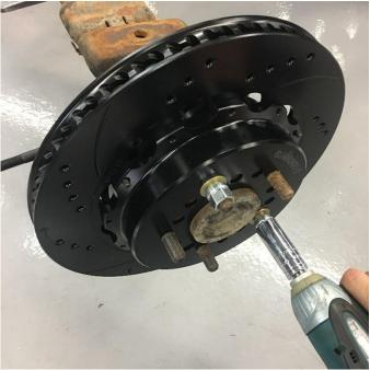
Arrange the rotor and hat in the position shown ensuring the arrow noting rotation direction is correct for its position on the vehicle. Start the first few threads of all 12 of the ¼-20 x .75 12-point bolts. Using an alternating sequence, apply red Loctite® 271 to the threads, and torque to **155 in-lbs**. The rotor can now be installed using 2 lug nuts to temporarily secure it. Make sure that there is no drag from the parking brake shoes on the rotor at this time.
