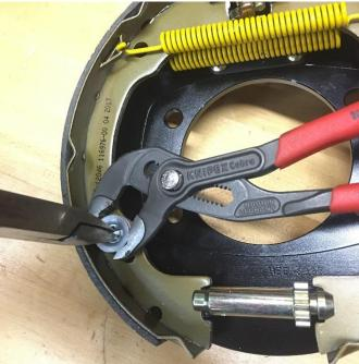
When using the stock parking brake cables, you will need to disassemble the parking brake assembly to install a new cable bracket. Your new levers are included separately. If you purchased our <u>Parking Brake Cable Kit</u>, steps 12-20 are **NOT** required. To swap them out, start by removing the retention springs as shown.
