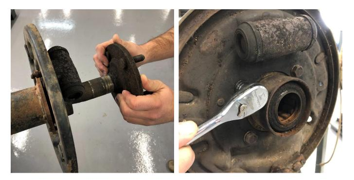
The axles will need to be removed from the housing by draining the fluid, then removing the differential cover, cross pin, and C-clip retainers. The 4 bolts retaining the drum backing plate to the axle can now be removed and discarded.
