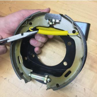
After installing the new bracket, you can now begin reassembly of the brake shoes. Start by installing the inside top retaining spring and assemble the shoes onto the backing plate. Then insert the tensioner and then install the outside top spring.
