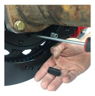
Adjust the parking brake shoes outward using a drum shoe adjustment tool (available at your local parts store) or a flat head screwdriver. You'll do this by spinning the rotor slowly until a slight drag is felt against the hat/drum. The rotor will need lug nuts installed while doing this so that is remains fully seated against the axle shaft.
