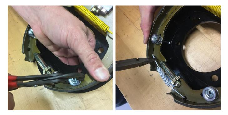
Reinstall the shoe retaining springs as shown, and then finish by reinstalling the bottom spring over the adjuster. At this time, the adjuster should be in the innermost position but not be bottomed out and difficult to adjust through the slotted window after assembly.
